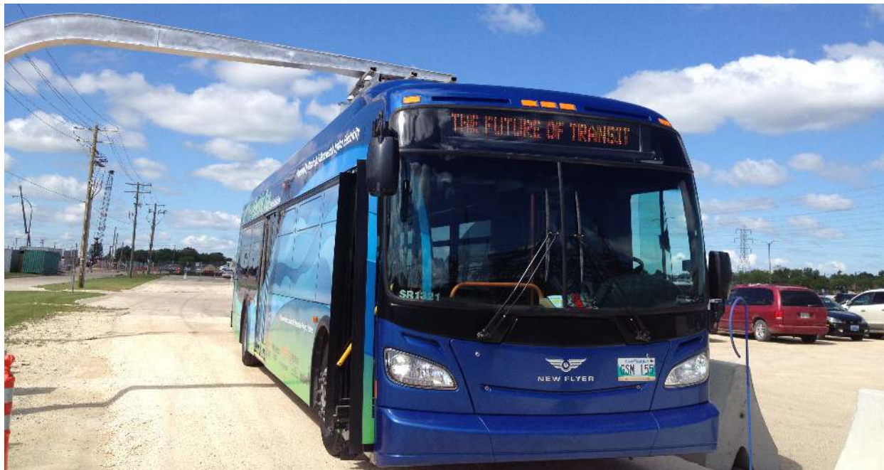
Figure 1. Photograph of prototype battery-electric bus during rapid charging event at Manitoba Hydro, Taylor Avenue temporary charging site, Winnipeg, Manitoba (July 2014 by R. Parsons)
