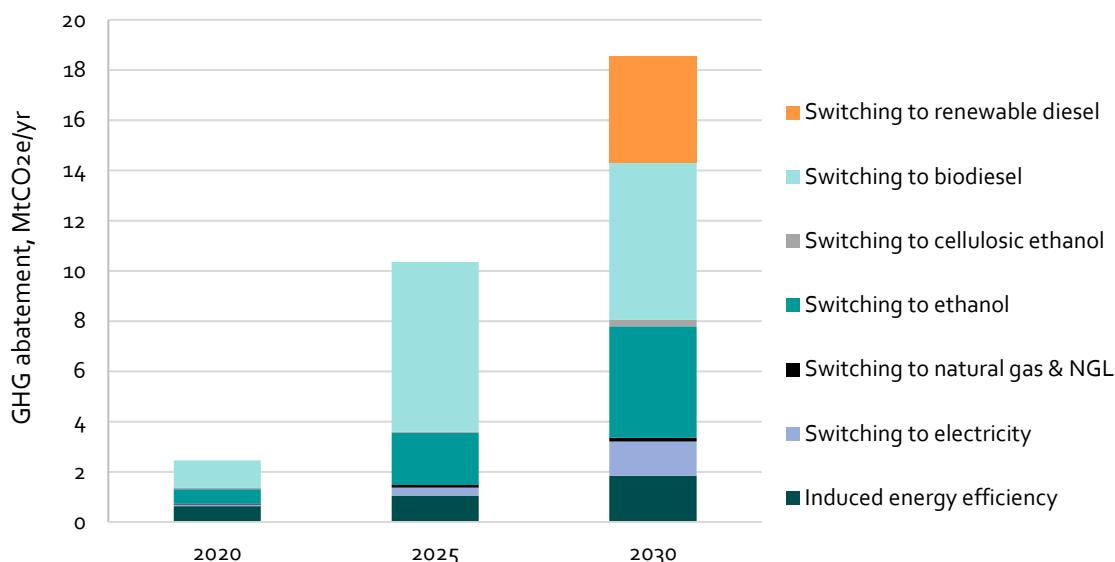
Figure 7: Abatement of transportation lifecycle GHG emissions by action, relative to the reference scenario
