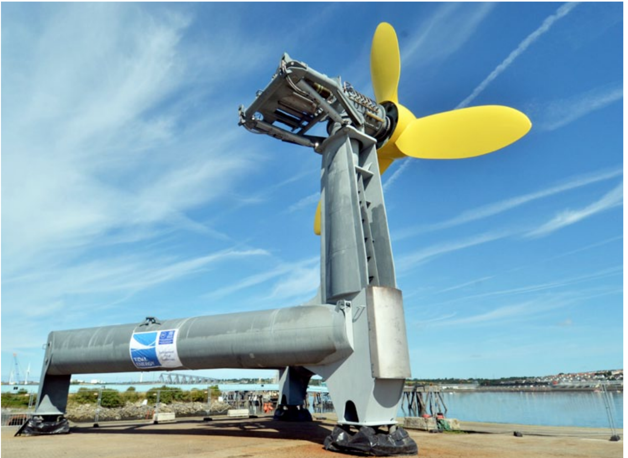
The 150-tonne "Spirit of the Sea" DeltaStream 400 kW tidal-energy generator will enter demonstration service this fall off the coast of Wales. Plans are underway for a 10 MW array of nine DeltaStream generators that would together power 10,000 homes.
