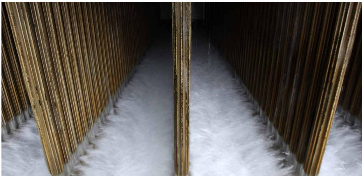
Sea water flows in an open rack type liquefied natural gas (LNG) vapourizer at Tokyo Gas Co.'s Sodegaura plant in Sodegaura City, Chiba Prefecture, Japan. Photo: Getty Images.
